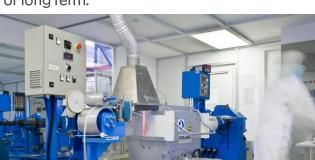
These production spaces with controled access are subject to regular particulate and bacteriological controls according to ISO 14 644 standard.
